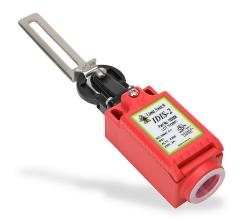
IDEM safety switch, lever hinge interlock, snap action, (1) N.C. safety output(s), plastic body, plastic head, (1) 1/2in NPT cable entry.
