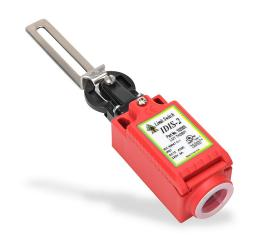
IDEM safety switch, lever hinge interlock, slow action, (3) N.C. safety output(s), plastic body, plastic head, (1) 1/2in NPT cable entry.
