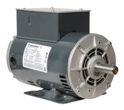
Marathon standard efficiency AC induction motor, general purpose, 2hp, 1-phase, 115/208-230 VAC, 1800rpm, ODP, NEMA 145T frame, rolled steel, rigid base mount.
