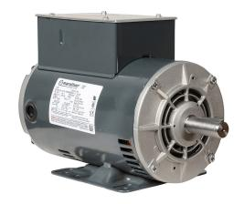
Marathon standard efficiency AC induction motor, general purpose, 2hp, 1-phase, 115/208-230 VAC, 1800rpm, ODP, 145T frame, rolled steel, rigid base mount.
