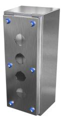
Hammond sanitary pushbutton enclosure, 4 holes, 30mm, slope top, NEMA 3R/4/4X/12,  $12 \times 5 \times 4in$  (HxWxD), wall mount, 304 stainless steel, #4 brush finish, screw cover.
