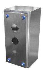
Hammond sanitary pushbutton enclosure, 3 holes, 30mm, slope top, NEMA 3R/4/4X/12,  $10 \times 5 \times 4$  in (HxWxD), wall mount, 304 stainless steel, #4 brush finish, screw cover.
