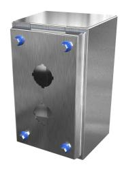
Hammond sanitary pushbutton enclosure, 2 holes, 30mm, slope top, NEMA 3R/4/4X/12, 8 x 5 x 4in (HxWxD), wall mount, 304 stainless steel, #4 brush finish, screw cover.
