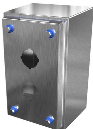
Hammond sanitary pushbutton enclosure, 2 holes, 30mm, slope top, NEMA 3R/4/4X/12, 8 x 5 x 4in (HxWxD), wall mount, 304 stainless steel, #4 brush finish, screw cover.
