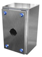
Hammond sanitary pushbutton enclosure, 1 hole, 30mm, slope top, NEMA 3R/4/4X/12, 8 x 5 x 4in (HxWxD), wall mount, 304 stainless steel, #4 brush finish, screw cover.
