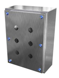
Hammond sanitary pushbutton enclosure, 6 holes, 22mm, slope top, NEMA 3R/4/4X/12, 12 x 9 x 4in (HxWxD), wall mount, 304 stainless steel, #4 brush finish, screw cover.
