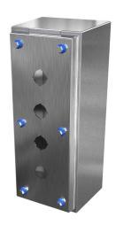
Hammond sanitary pushbutton enclosure, 4 holes, 22mm, slope top, NEMA 3R/4/4X/12, 12 x 5 x 4in (HxWxD), wall mount, 304 stainless steel, #4 brush finish, screw cover.
