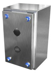
Hammond sanitary pushbutton enclosure, 2 holes, 22mm, slope top, NEMA 3R/4/4X/12, 8 x 5 x 4in (HxWxD), wall mount, 304 stainless steel, #4 brush finish, screw cover.
