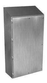
Hammond Waterfall series enclosure, slope top, NEMA 3R/4/4X/12/13,  $60 \times 36 \times 16$  in (HxWxD), wall mount, 304 stainless steel, #4 brush finish, single-door, 1/4-turn semi-flush stainless steel.
