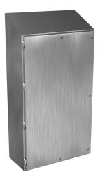
Hammond Waterfall series enclosure, slope top, NEMA 3R/4/4X/12/13, 60 x 36 x 16in (HxWxD), wall mount, 304 stainless steel, #4 brush finish, single-door, 1/4-turn semi-flush stainless steel.
