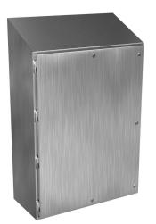
Hammond Waterfall series enclosure, slope top, NEMA 3R/4/4X/12/13, 48 x 36 x 16in (HxWxD), wall mount, 304 stainless steel, #4 brush finish, single-door, 1/4-turn semi-flush stainless steel.
