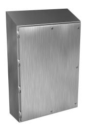
Hammond Waterfall series enclosure, slope top, NEMA 3R/4/4X/12/13,  $48 \times 36 \times 12$  in (HxWxD), wall mount, 304 stainless steel, #4 brush finish, single-door, 1/4-turn semi-flush stainless steel.
