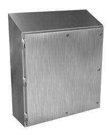
Hammond Waterfall series enclosure, slope top, NEMA 3R/4/4X/12/13,  $36 \times 36 \times 12$  in (HxWxD), wall mount, 304 stainless steel, #4 brush finish, single-door, 1/4-turn semi-flush stainless steel.
