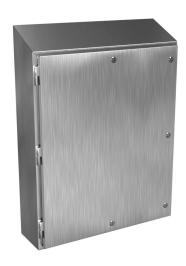
Hammond Waterfall series enclosure, slope top, NEMA 3R/4/4X/12/13,  $36 \times 30 \times 8$  in (HxWxD), wall mount, 316 stainless steel, #4 brush finish, single-door, 1/4-turn semi-flush stainless steel.
