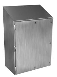
Hammond Waterfall series enclosure, slope top, NEMA 3R/4/4X/12/13, 36 x 30 x 16in (HxWxD), wall mount, 304 stainless steel, #4 brush finish, single-door, 1/4-turn semi-flush stainless steel.
