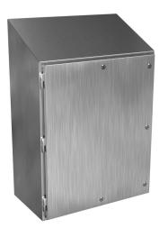
Hammond Waterfall series enclosure, slope top, NEMA 3R/4/4X/12/13, 36 x 30 x 16in (HxWxD), wall mount, 316 stainless steel, #4 brush finish, single-door, 1/4-turn semi-flush stainless steel.
