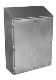
Hammond Waterfall series enclosure, slope top, NEMA 3R/4/4X/12/13,  $36 \times 30 \times 12$  in (HxWxD), wall mount, 304 stainless steel, #4 brush finish, single-door, 1/4-turn semi-flush stainless steel.
