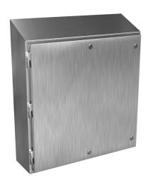
Hammond Waterfall series enclosure, slope top, NEMA 3R/4/4X/12/13,  $30 \times 30 \times 8$  in (HxWxD), wall mount, 316 stainless steel, #4 brush finish, single-door, 1/4-turn semi-flush stainless steel.
