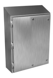
Hammond Waterfall series enclosure, slope top, NEMA 3R/4/4X/12/13,  $30 \times 24 \times 8$  in (HxWxD), wall mount, 304 stainless steel, #4 brush finish, single-door, 1/4-turn semi-flush stainless steel.
