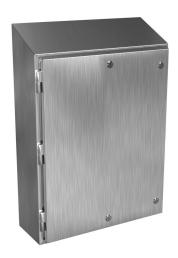
Hammond Waterfall series enclosure, slope top, NEMA 3R/4/4X/12/13,  $30 \times 24 \times 8$  in (HxWxD), wall mount, 316 stainless steel, #4 brush finish, single-door, 1/4-turn semi-flush stainless steel.
