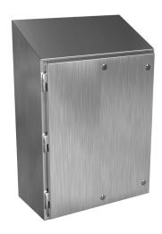
Hammond Waterfall series enclosure, slope top, NEMA 3R/4/4X/12/13,  $30 \times 24 \times 12$ in (HxWxD), wall mount, 304 stainless steel, #4 brush finish, single-door, 1/4-turn semi-flush stainless steel.
