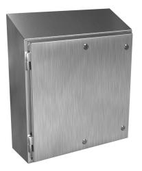
Hammond Waterfall series enclosure, slope top, NEMA 3R/4/4X/12/13, 24 x 24 x 8in (HxWxD), wall mount, 304 stainless steel, #4 brush finish, single-door, 1/4-turn semi-flush stainless steel.
