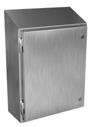
Hammond Waterfall series enclosure, slope top, NEMA 3R/4/4X/12/13, 24 x 20 x 8in (HxWxD), wall mount, 304 stainless steel, #4 brush finish, single-door, 1/4-turn semi-flush stainless steel.
