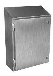
Hammond Waterfall series enclosure, slope top, NEMA 3R/4/4X/12/13,  $24 \times 20 \times 8$ in (HxWxD), wall mount, 316 stainless steel, #4 brush finish, single-door, 1/4-turn semi-flush stainless steel.
