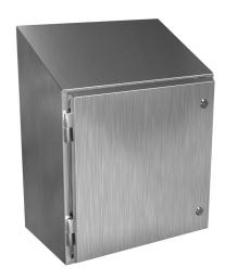
Hammond Waterfall series enclosure, slope top, NEMA 3R/4/4X/12/13,  $20 \times 20 \times 12$  in (HxWxD), wall mount, 316 stainless steel, #4 brush finish, single-door, 1/4-turn semi-flush stainless steel.
