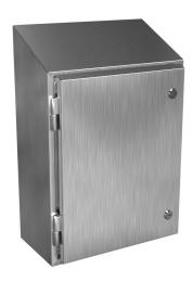
Hammond Waterfall series enclosure, slope top, NEMA 3R/4/4X/12/13,  $20 \times 16 \times 8$  in (HxWxD), wall mount, 304 stainless steel, #4 brush finish, single-door, 1/4-turn semi-flush stainless steel.
