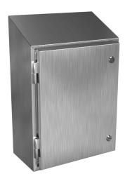
Hammond Waterfall series enclosure, slope top, NEMA 3R/4/4X/12/13,  $20 \times 16 \times 8$  in (HxWxD), wall mount, 316 stainless steel, #4 brush finish, single-door, 1/4-turn semi-flush stainless steel.
