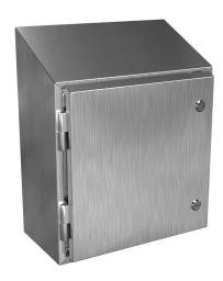
Hammond Waterfall series enclosure, slope top, NEMA 3R/4/4X/12/13,  $16 \times 16 \times 8$  in (HxWxD), wall mount, 304 stainless steel, #4 brush finish, single-door, 1/4-turn semi-flush stainless steel.
