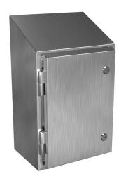
Hammond Waterfall series enclosure, slope top, NEMA 3R/4/4X/12/13,  $16 \times 12 \times 8$  in (HxWxD), wall mount, 304 stainless steel, #4 brush finish, single-door, 1/4-turn semi-flush stainless steel.
