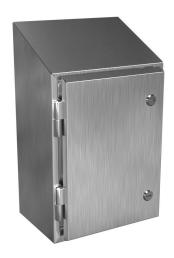
Hammond Waterfall series enclosure, slope top, NEMA 3R/4/4X/12/13,  $16 \times 12 \times 8$  in (HxWxD), wall mount, 316 stainless steel, #4 brush finish, single-door, 1/4-turn semi-flush stainless steel.
