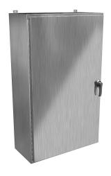
Hammond enclosure, NEMA 3R/4/4X/12/13, 60 x 36 x 16in (HxWxD), wall mount, 304 stainless steel, #4 brush finish, single-door, 3-point 316 stainless steel padlocking handle.
