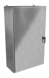
Hammond enclosure, NEMA 3R/4/4X/12/13, 60 x 36 x 16in (HxWxD), wall mount, 316 stainless steel, #4 brush finish, single-door, 3-point 316 stainless steel padlocking handle.
