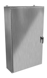
Hammond enclosure, NEMA 3R/4/4X/12/13, 60 x 36 x 12in (HxWxD), wall mount, 304 stainless steel, #4 brush finish, single-door, 3-point 316 stainless steel padlocking handle.
