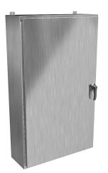
Hammond enclosure, NEMA 3R/4/4X/12/13, 60 x 36 x 12in (HxWxD), wall mount, 316 stainless steel, #4 brush finish, single-door, 3-point 316 stainless steel padlocking handle.
