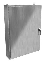
Hammond enclosure, NEMA 3R/4/4X/12/13, 48 x 36 x 8in (HxWxD), wall mount, 304 stainless steel, #4 brush finish, single-door, 3-point 316 stainless steel padlocking handle.
