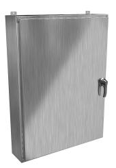
Hammond enclosure, NEMA 3R/4/4X/12/13, 48 x 36 x 8in (HxWxD), wall mount, 316 stainless steel, #4 brush finish, single-door, 3-point 316 stainless steel padlocking handle.
