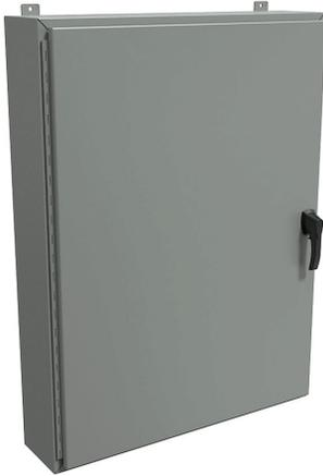
Hammond enclosure, NEMA 3R/4/12, 48 x 36 x 8in (HxWxD), wall mount, carbon steel, ANSI 61 gray, powder coat finish, single-door, 3-point padlocking handle.
