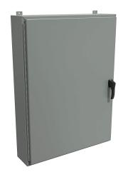
Hammond enclosure, NEMA 3R/4/12, 48 x 36 x 8in (HxWxD), wall mount, carbon steel, ANSI 61 gray, powder coat finish, single-door, 3-point padlocking handle.
