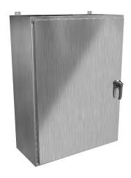
Hammond enclosure, NEMA 3R/4/4X/12/13, 48 x 36 x 16in (HxWxD), wall mount, 316 stainless steel, #4 brush finish, single-door, 3-point 316 stainless steel padlocking handle.
