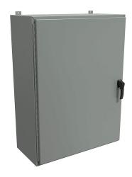
Hammond enclosure, NEMA 3R/4/12, 48 x 36 x 16in (HxWxD), wall mount, carbon steel, ANSI 61 gray, powder coat finish, single-door, 3-point padlocking handle.
