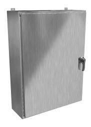
Hammond enclosure, NEMA 3R/4/4X/12/13, 48 x 36 x 12in (HxWxD), wall mount, 316 stainless steel, #4 brush finish, single-door, 3-point 316 stainless steel padlocking handle.
