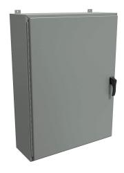
Hammond enclosure, NEMA 3R/4/12, 48 x 36 x 12in (HxWxD), wall mount, carbon steel, ANSI 61 gray, powder coat finish, single-door, 3-point padlocking handle.
