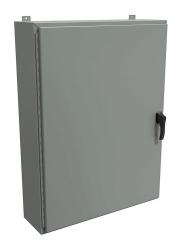
Hammond enclosure, NEMA 3R/4/12, 48 x 36 x 10in (HxWxD), wall mount, carbon steel, ANSI 61 gray, powder coat finish, single-door, 3-point padlocking handle.
