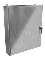
Hammond enclosure, NEMA 3R/4/4X/12/13, 42 x 36 x 8in (HxWxD), wall mount, 304 stainless steel, #4 brush finish, single-door, 3-point 316 stainless steel padlocking handle.
