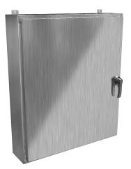
Hammond enclosure, NEMA 3R/4/4X/12/13, 42 x 36 x 8in (HxWxD), wall mount, 316 stainless steel, #4 brush finish, single-door, 3-point 316 stainless steel padlocking handle.
