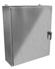
Hammond enclosure, NEMA 3R/4/4X/12/13, 42 x 36 x 12in (HxWxD), wall mount, 316 stainless steel, #4 brush finish, single-door, 3-point 316 stainless steel padlocking handle.
