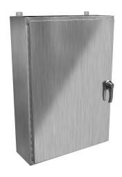
Hammond enclosure, NEMA 3R/4/4X/12/13, 42 x 30 x 10in (HxWxD), wall mount, 304 stainless steel, #4 brush finish, single-door, 3-point 316 stainless steel padlocking handle.
