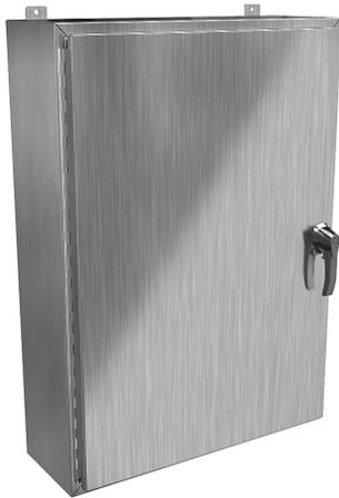
Hammond enclosure, NEMA 3R/4/4X/12/13, 42 x 30 x 10in (HxWxD), wall mount, 304 stainless steel, #4 brush finish, single-door, 3-point 316 stainless steel padlocking handle.
