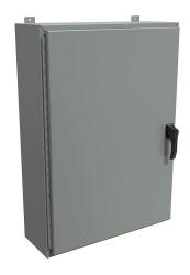
Hammond enclosure, NEMA 3R/4/12, 42 x 30 x 10in (HxWxD), wall mount, carbon steel, ANSI 61 gray, powder coat finish, single-door, 3-point padlocking handle.
