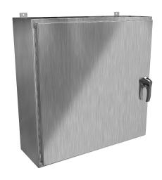
Hammond enclosure, NEMA 3R/4/4X/12/13, 36 x 36 x 12in (HxWxD), wall mount, 304 stainless steel, #4 brush finish, single-door, 3-point 316 stainless steel padlocking handle.
