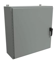
Hammond enclosure, NEMA 3R/4/12, 36 x 36 x 12in (HxWxD), wall mount, carbon steel, ANSI 61 gray, powder coat finish, single-door, 3-point padlocking handle.
